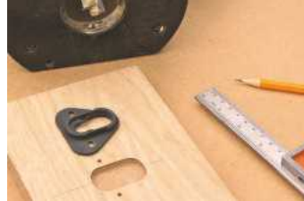
With the aid of a router the gap made by surface mounting can be reduced
